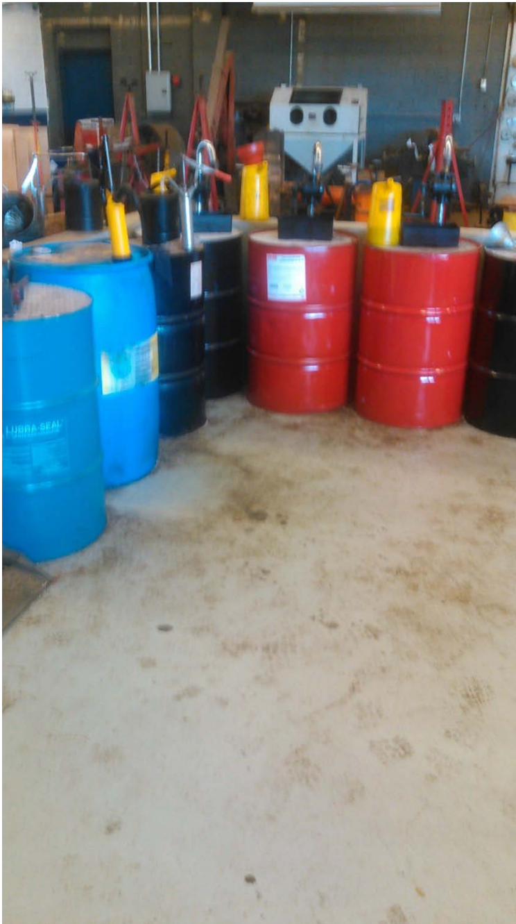
BMP Highway Maintenance Garage Properly contained drum storage in 110% Containment diked area
